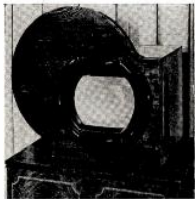
CROSLY'S color converter which was demonstrated to New York dealers and newsmen fortnight ago [BROADCASTING • TELECASTING, July 2]. The converter is tuned through the standard receiver, Crosley explains, but separate dials on the right are used to control color brightness, focus hold and contrast. The unit uses a 10-inch screen with a magnifier, which brings the color picture up to 12½-inch size. Converters will be put into production when public demand and hours of color telecasting warrant the move, Crosley officials said.
